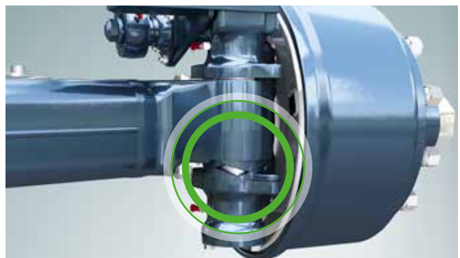
Steering housing when cornering (up to 27 degrees, depending on vehicle model)
