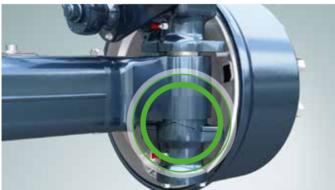
Steering housing when driving straight ahead (zero position)
