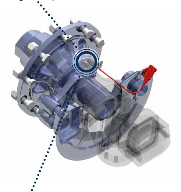
speed sensor with detection of rotating direction
