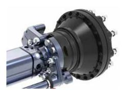
Can be combined with any suspension system thanks to varying brake camshaft position.
